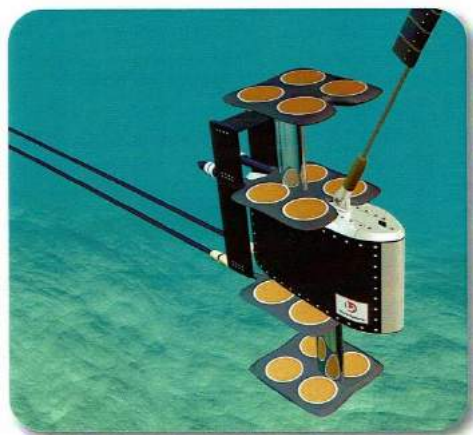
Unique extension/retraction mechanism transforms compact tow-body configuration to a large-aperture multidirectional transmitter.
